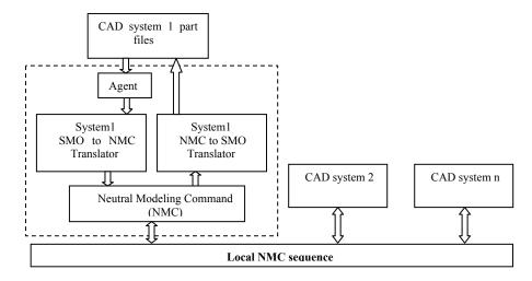
Fig. 1. The procedural CAD model exchange platform
