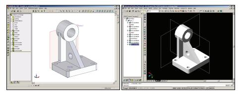
Fig. 7. View of the source SolidWorks part file Fig. 8. View of the destination MDT part file
